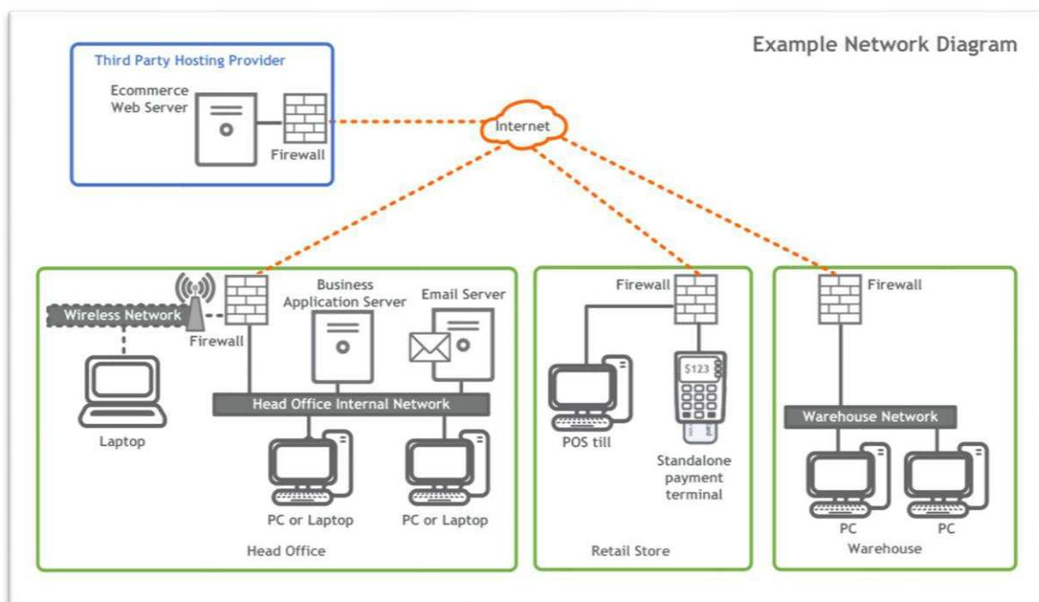
2. Create a copy of the network diagram for each payment channel that is used – Ecommerce, Face-to-face, and MOTO. A single diagram can work for smaller configurations but may become confusing with multi-channel environments.
